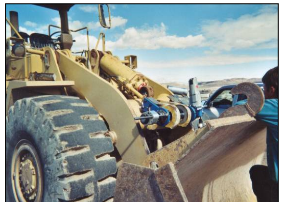
Line Boring Of A Digger Bucket Pivot Point
