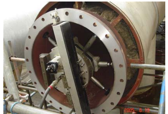
2M Ø Flange Being Machined Perfectly Flat
