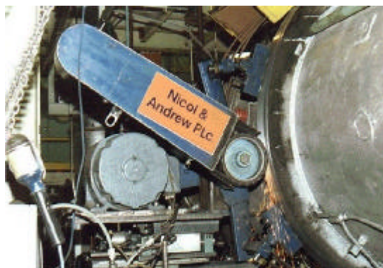
Grinding a 3M diameter Kiln Tyre
