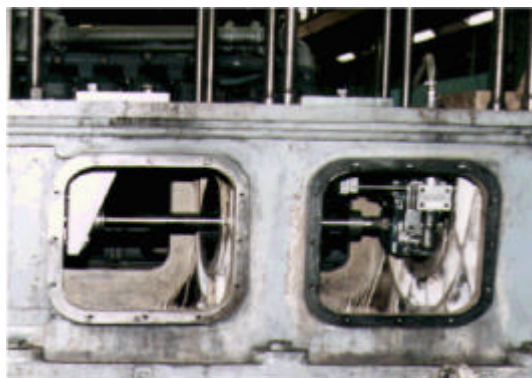
On Site Line Boring of a 380mm Ø Diesel Engine Block
