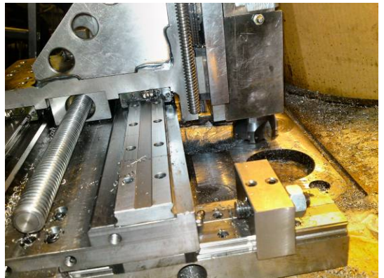
On Site Milling Of A Diesel Engine Entablature Base
