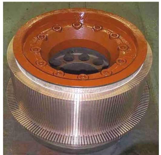
An Example of a Machined Commutator
