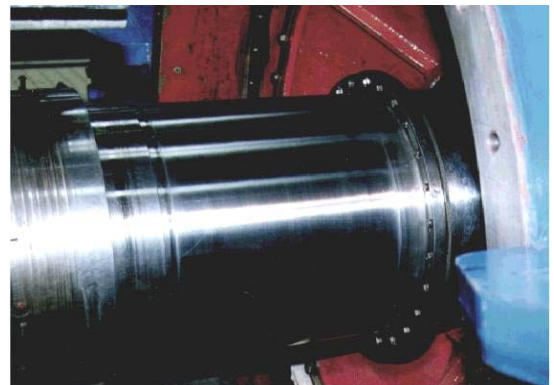
A 533 mm \varnothing Turbine Journal AFTER Machining and Polishing
