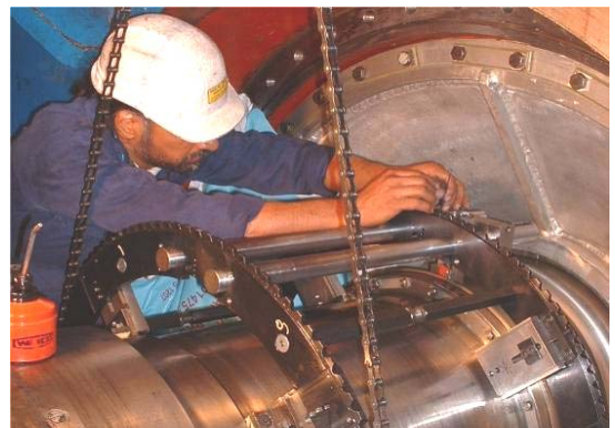
Machining and Polishing of a 610 mm \varnothing Hydrogen Seal Face
